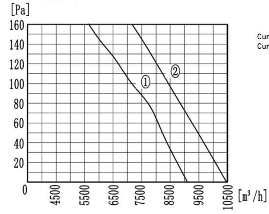
Curve 1: 50HZ Curve 2: 60HZ
